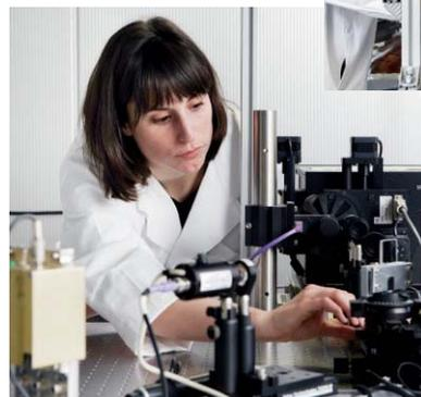
A spectroscopic goniometry system enables the measurement of directional and spectral radiative properties of semi-transparent media, such as complex porous materials applied in thermal and thermochemical energy conversion processes.
