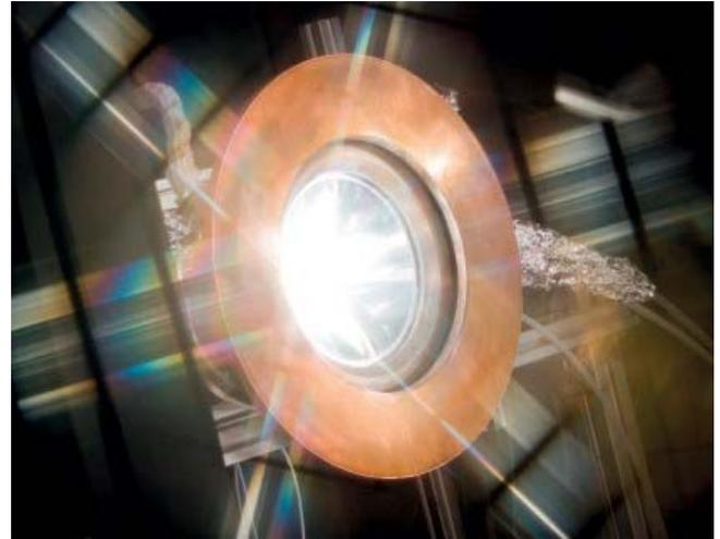
A solar thermochemical reactor prototype for splitting H<sub>2</sub>O and CO<sub>2</sub> via redox cycles, exposed to concentrated solar radiation.
