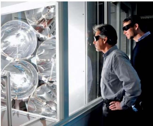
Experimentation at the High-Flux Solar Simulator: solar thermal receivers and thermochemical reactors are subjected to high radiative fluxes (> 5,000 suns), and tested at high temperatures (> 1000°C) and heating rates (> 1000°C/s), under similar radiative heat transfer characteristics of highly concentrating solar systems.
