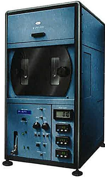
Figure 3.9: Photograph of the VTI-SA+ Vapour Sorption Analyser, with its control panel.
