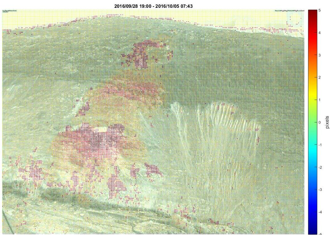
**Figure 2:** Surface deformation obtained by analyzing digital photos acquired from the Driest location
