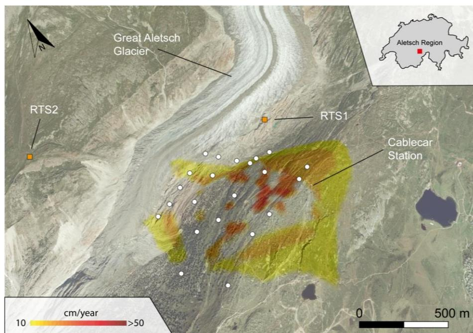
**Figure 1:** Surface deformation at Moosfluh retrieved with the analysis of space borne SAR data and the Total Station (RTS) monitoring network. Location for the installation of the Raspberry Shakes seismometers will be at the RTS locations + at the Moosfluh cable car station.
