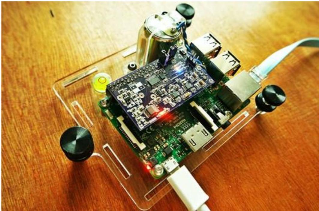
**Figure 3:** Raspberry shake seismometer ([www.raspberrypi.org](http://www.raspberrypi.org))
