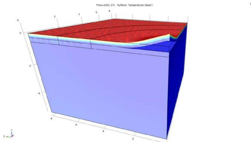
3D model developed in COMSOL Multiphysics correlates hourly bedrock temperature fluctuations with the buckling of a 0.5 m thick bedrock slab.
