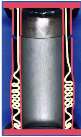
Figure 6 Yielding support with LSC elements incorporated in the shotcrete lining and between steel sets with yielding couplings [12].
