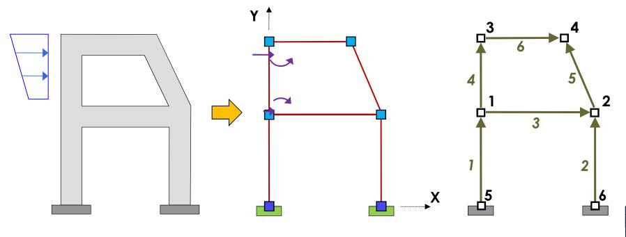
Global coordinate system Nodes Elements Boundary conditions Loads
