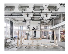
A project member manually bolts the timber beams together that have been jointly preplaced by the two robots.
