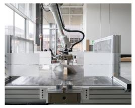
One of the robots taking a timber beam to the saw in order for it to be cut to size.
