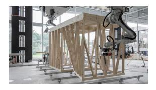
One of a total of six spatial, geometrically unique timber modules prefabricated with the novel robotbased building method "Spatial Timber Assemblies".
