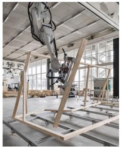
Highly precise robotic positioning of a timber beam according to the computational design.
