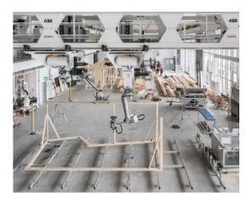
The Robotic Fabrication Laboratory of ETH Zurich is the world's first research platform for large-scale robotic prefabrication in architecture.
