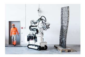
The In situ Fabricator equipped with the Mesh Mould toolhead and the Mesh Mould prototype with a double-curved geometry at the Robotic Fabrication Laboratory, ETH Zurich.
