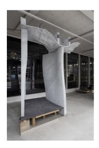
DFAB HOUSE prototype at the Robotic Fabrication Laboratory, ETH Zurich. The prototype demonstrates the seamless combination of other innovation objects on the DFAB HOUSE, such as Smart Dynamic Casting and the Smart Slab with the Mesh Mould wall.
