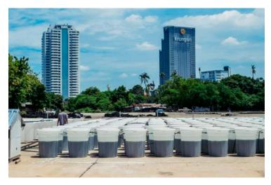
The intended Life Expectancy of the spirulina production system is a minimum of 5-years. Some components will last longer than this while will have a shorter life span and are intended to be replaced as part of the routine system maintenance when necessary. Additionally, because our design relies on the injection of forced air for aeration and mixing, we are able to utilize CO2 emissions from industrial sites as an option, reducing the carbon footprint of our customers.
