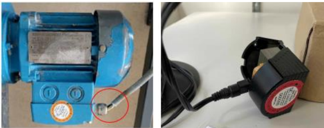
Cable is pulled out and housing is defective: frequently observed defects. Images: E+S.
