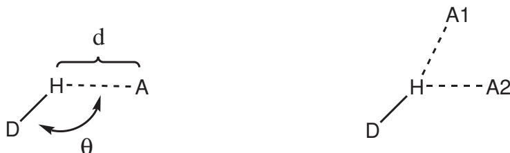
FIGURE 20.1. Left: definition of a hydrogen bond using a maximum distance d(\text{H-A}) and a minimum angle \theta(\text{D-H-A}) . Right: a three-centre hydrogen bond is defined by the additional specification of a minimum value for the sum of the three angles \theta(\text{D-H-A1}) , \theta(\text{D-H-A2}) and \theta(\text{A1-H-A2}) , and a maximum value for the (improper) dihedral angle \varphi(\text{H-A2-A1-D}) .
