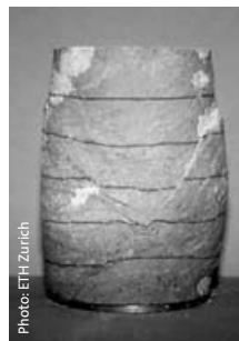
A kakirite sample severely deformed after testing.
