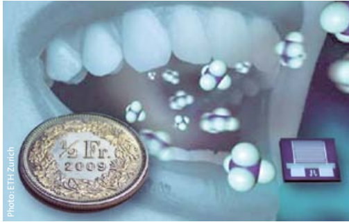
The sensor detects acetone molecules from the mouth.
